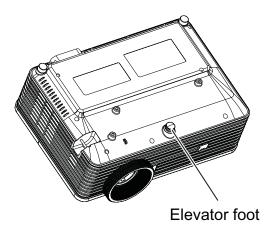
The projector is equipped with an elevator foot to adjust the image height. To raise or lower the image, turn the elevator foot to fine-tune the height.
