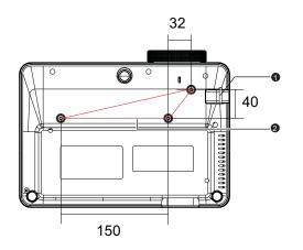
Ceiling mount screws: M4 x 8 (Max. L = 8 mm)
