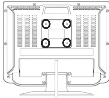
**Important – Ensure the length of screws included with your wall mount that secure the Wall Mount to the TV do not exceed 8mm. Using longer screws could cause irreparable damage to the TV**
