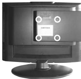
**Important – Ensure the length of screws included with your wall mount that secure the Wall Mount to the TV do not exceed 10 mm. Using longer screws could cause irreparable damage to the TV**
