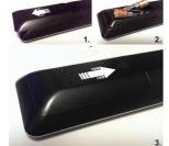
Remove the back cover to reveal the battery compartment and make sure the batteries are inserted the right way round. Suitable battery types for this remote are AAA, IEC R03 1.5V.
