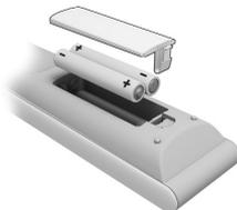
Remove the back cover to reveal the battery compartment and make sure the batteries are inserted the right way round. Suitable battery types for this remote are AAA, IEC R03 1.5V.
