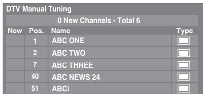
When the multiplex is found any channels that are not currently in the channel list will be added and the channel information at the top of the screen will be updated.
