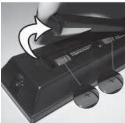
Remove the back cover to reveal the battery compartment and make sure the batteries are inserted the right way round. Suitable battery types for this remote are AAA, IEC R03 1.5V.
