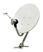
The LNB (Low Noise Block converter) is used to take a wide band of relatively high frequencies, amplify and convert them to similar signals that is carried at a much lower frequency, which is called Intermediate Frequency (IF).
