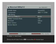
To use the DiSEqC 1.2 protocol, select the Installation > Motorized DiSEqC 1.2 menu. You should see a screen like the left figure.
