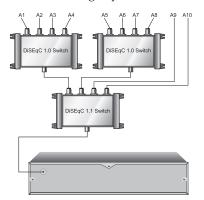
For example, to select the antenna connected to the A5 input in the left figure, set the DiSEqC 1.1 option to 2 of 4 and the DiSEqC 1.0 option to 1 of 4. If you have a mini DiSEqC 1.0 switch which has only two inputs, you should set the DiSEqC 1.0 option to Mini A instead of 1 of 4.
