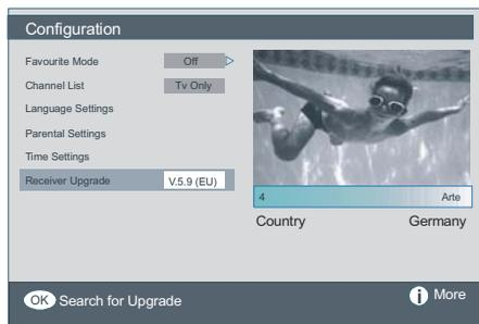
In the configuration menu, highlight the “**Receiver Upgrade**” item by pressing **▲** or **▼** buttons and press “**OK**” button to start upgrade process. The following menu appears on the screen.
