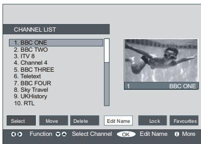
Now pressing **◀** or **▶** buttons moves to the previous/next character. Pressing **▲** or **▼** buttons toggles the current character, i.e., ‘b’ character becomes ‘a’ on **▼** and ‘c’ on **▲**. Pressing the numeric buttons ‘0...9’ replaces the highlighted character with the characters printed above the key one by one as the button is pressed.
