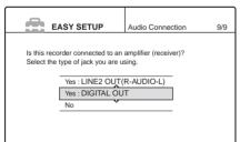
**19** Press  $\uparrow/\downarrow$  to select the type of jack (if any) you are using to connect to an amplifier (receiver), then press ENTER.
