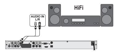
Connect the audio output sockets L/R on the rear panel of the DVD player to the corresponding audio inputs on the HiFi system with an audio cinch cable.
