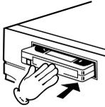
Insert the cassette tape with its labeled side facing up and the erase prevention tab positioned at your left. An inverted cassette tape cannot be inserted.
