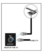
• Connect the aerial or cable TV plug to the RF input socket located at the rear of the TV and connect the cable plug coming out from the TV out socket located on the devices (VCR, DVB etc.) to this socket as well.
