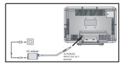
IMPORTANT: The TV set is designed to operate on 24V DC. For this, an adaptor is used which gives 24V DC voltage. Connect this adaptor to a system that supplies 230V AC, 50 Hz.
