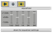
Press "▼" button to select the first frequency band. Press "◀" / "▶" button to select the other frequency bands. Selected band can be adjusted by pressing "▲" / "▼" button.
