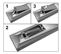
**NOTE:** Remove the batteries from remote control handset when it is not to be used for a long period.Otherwise it can be damaged due to any leakage of batteries.
