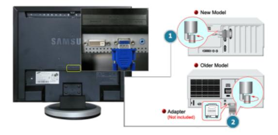
Using the D-sub (Analog) connector on the video card.
