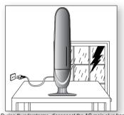
During thunderstorms, disconnect the AC main plug from the wall outlet. Voltage peaks due to lightning could damage the unit.
