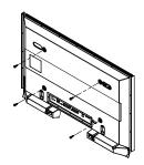
Tighten the screws of the plastic hanger (shown in picture 2) to the back side of the PDP.
