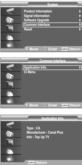
This contains information on CAM inserted in the CI slot and displays it.
