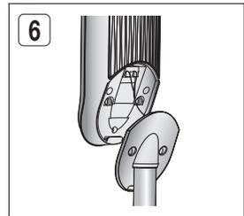
7. Fully insert the Stand Bracket into the speaker's clasp to stand speaker.
