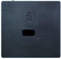
The Kensington lock is a device used to physically fix the system when using it in a public place. (The locking device has to be purchased separately.)
