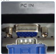
Computer Connection Terminal (15 Pin D-SUB)
