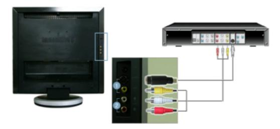
1. Input devices such as DVD, VCR or Camcorder are connected to the Video or S-Video terminal of the monitor using the S-Video cable.
