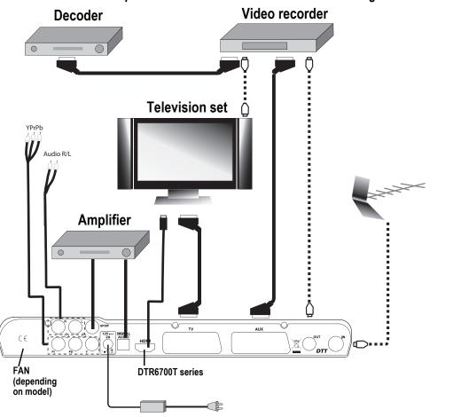
Connecting auxiliary equipment (e.g. a video recorder) for a television set with a Scart socket.
