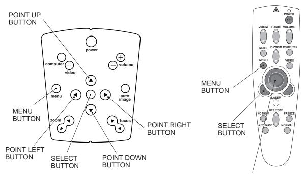
POINT (UP/DOWN/LEFT/RIGHT) BUTTON Pressing the button upward, downward, leftward or rightward.
