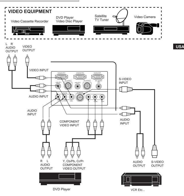
**NOTE:** When connecting the cable, the power cords of both the projector and the external equipment should be disconnected from AC outlet. Turn the projector on before the peripheral equipment is switched on.
