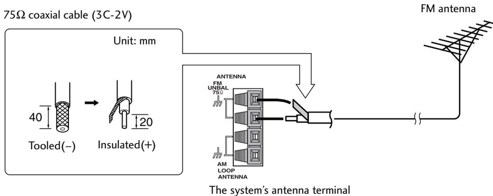
**Note:** The ground mark (⏏) on the antenna terminal refers to measures to reduce reception noise when an antenna is connected. It does not refer to a safety ground.
