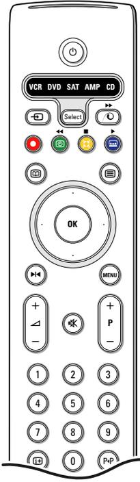
This system remote control operates the following Philips equipment: TV, VCR, DVD, DVD/R, SAT (RC5/RC6), AMP (+TUNER), CD, CD/R.
