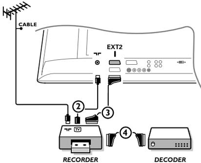
Connect the aerial cables ①, ② and, to obtain the optimum picture quality, eurocable ③ as shown. If your recorder does not have a euroconnector, the only possible connection is via the aerial cable. You will therefore need to tune in your recorder's test signal and assign it programme number 0 or store the test signal under a programme number between 90 and 99, see Manual installation, p. 6. See the handbook of your recorder.
