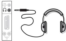
When headphones are connected, the sound on the TV set will be cut. The **P** keys are used to adjust the volume level. The headphone impedance must be between 32 and 600 Ohms.
