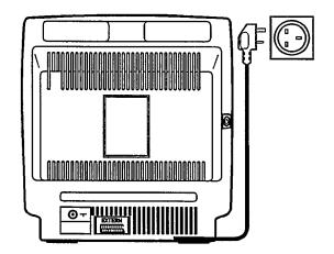
2 Switch the set on. The power switch is located on the left side panel of the set.
