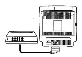
1 Connect the decoder to the set with a scart cable (EXTERNAL) socket).
