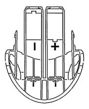
3 Close the battery compartment, by sliding it onto the remote control, until you hear a 'click'.
