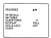
With the or the menu button you can determine the minutes left until switch off in 15 minutes intervals.
