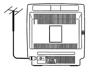
2 If you use the auxiliary aerial supplied, push the aerial into the mounting on the back panel until it snaps into place. Pull out he telescopic rod(s) as far as required. Tilt and rotate the aerial until you have got the best picture quality. Rotate the aerial until you have got the best picture quality.
