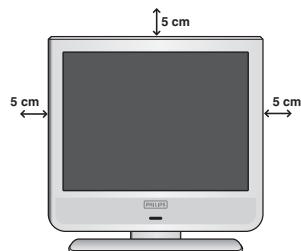
Place your TV on a solid stable surface. To avoid danger do not expose the TV to water, or a heat source (e.g. lamp, candle, radiator). Do not obstruct the ventilation grid at the rear.
