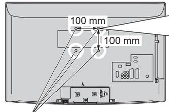
Holes for wall-hanging bracket installation
