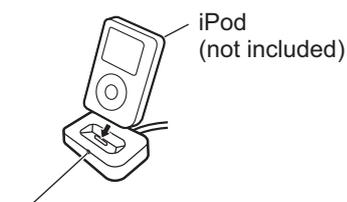
The indicator lights up when the iPod is inserted, and charging begins.
