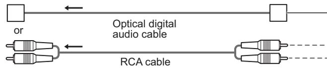
To enjoy the sound from the external equipment in multi-channel sound (e.g. Dolby Digital 5.1ch), connect the equipment to the amplifier. For the connections, read the manuals of the equipment and amplifier.
