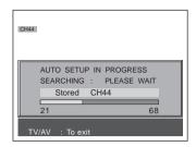
First, ensure that the recording device is in Standby mode. If the TV has not been programmed for you then **Auto setup** will begin, your stations will be located, sorted into order and stored ready for use (refer to page 17).
