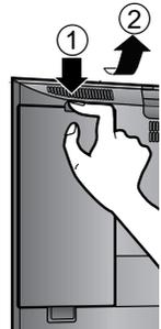
1. Disengage the claws at the uppermost end.
