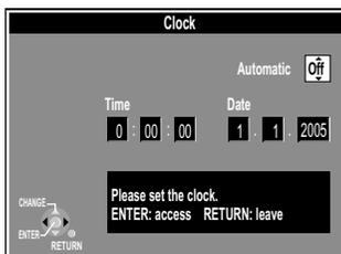
If Clock setting is set to AUTO, do not set it to MANUAL, otherwise the automatic time correction function is deactivated.
