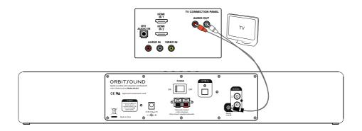
Use the included analogue RCA/Jack cable to connect the audio output from your TV to the soundbar.
