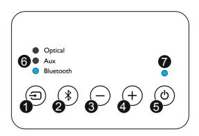
1. Source: Press to cycle through the inputs. This controls what device is
