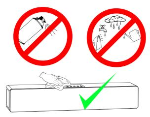
Use a soft, clean cloth moistened with plain, luke-warm water to clean the exterior of the unit. Glass cleaner is a good way to remove finger marks, but please use it sparingly, and avoid contact with the actual loudspeaker driver units.
