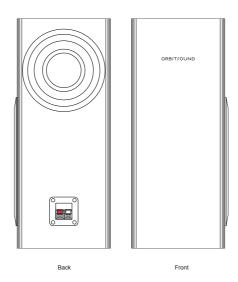
The subwoofer is a wired passive loudspeaker that produces powerful Hi-Fi bass. It has been designed specially to complement the soundbar.
