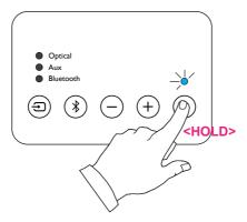
You may wish to reset the soundbar settings. To do this, switch the unit on, then press and hold the power button for a few seconds on the control panel. The soundbar status light will flash, and then the soundbar will reset. Optical source will be selected with default settings.
