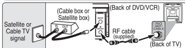
Select this connection when you want to view or record a scrambled channel. With this connection, channels cannot be changed on the unit. You can view or record ONLY the channels you have selected on the cable box or the satellite box.
