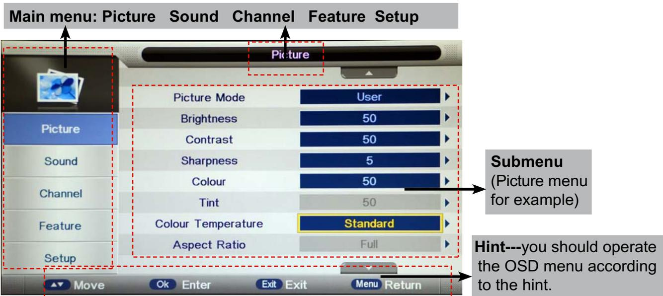
Use  $\wedge/\vee$  button to select the main menu, and press  $>/\text{OK}$  button to enter the submenu. In the submenu, use  $\wedge/\vee$  button to select the function item, press  $>/\text{OK}$  button to enter the setup menu, then press  $</>$  button to adjust, or press  $\wedge/\vee$  to select and press **OK** /  $</>$  button to confirm.
