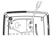
**WARNING**: To avoid burns, allow the projector to cool for at least 60 minutes before you replace the lamp.
