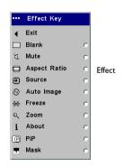
**PiP**: (Picture in Picture) allows you to overlay a smaller window showing the video source on top of the larger computer source window. You must have both a computer and video source connected to use PIP. You can't show a computer image in the smaller PiP window, only a video image. You can select a small, medium, or large window. You can also move the PiP window on the screen using the PiP Position X and Y options in the menu. Press the up and down arrows to change the position.
