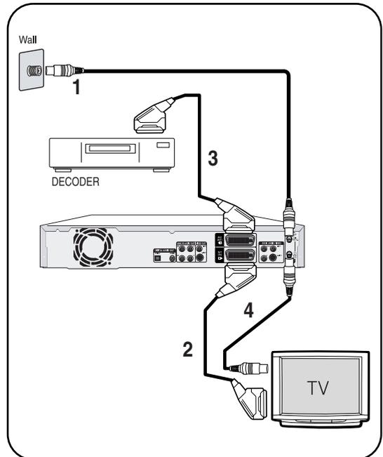
1. Connect RF antenna cables as shown.
