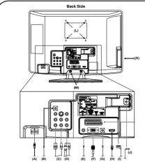
(A) Power supply: Connect the supplied power cable to an AC 220-240V/50Hz mains power supply only - do not attempt to connect it to any other type of supply. Never try to repair a damaged AC power cord with
