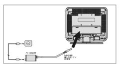
IMPORTANT: The TV set is designed to operate on 12 V DC. For this, an adaptor is used which gives 12V DC voltage. Connect this adaptor to a system that supplies 220-240 V AC, 50 Hz.
