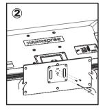
Insert base, then 3 screws (provided) and fasten securely. Please fasten with cross screwdriver.
