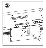
Insert base, then 4 screws (provided) and fasten securely. Please fasten with cross screwdriver.
