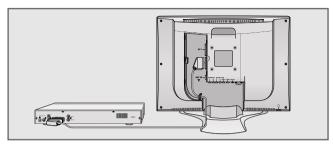
1 Connect the »AV1« or »AV2« socket (Amira 17 and 20 only) on the television and the corresponding socket on the video recorder, DVD player or the set-top box with a Euro-AV (Scart) cable.
