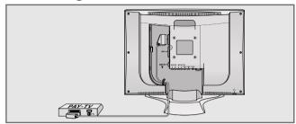
1 Connect the »AV1« socket on the television set and the appropriate socket on the decoder using a EURO-AV cable.
