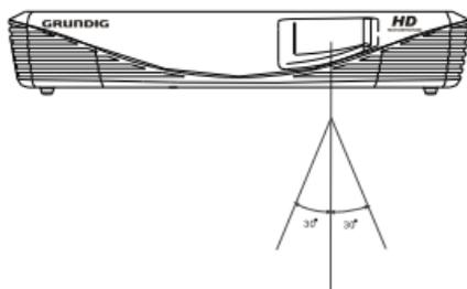
The Remote Control will not operate if its path is blocked.
