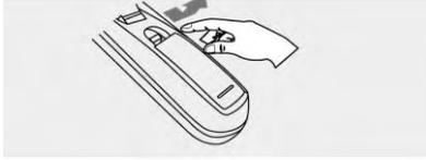
2. Install the batteries into the battery tray.
