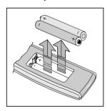
**NOTE:** Remove batteries from remote control handset when it is not to be used for a long period. Otherwise it can be damaged due to any leakage of batteries.
