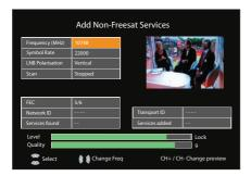
Using the arrow and number buttons, select and enter the frequency, symbol rate and LNB polarisation.
