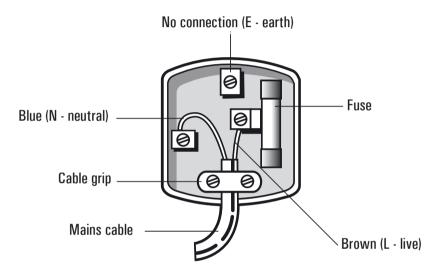
The colours of the wires in the receiver's power lead may not match the coloured markings in your plug, so you should follow these instructions.
