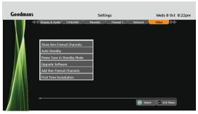
**Show Non Freesat Channels** - This setting allows you to see the manually added free to air channels in the channel list.
