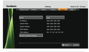
**DON'T FORGET!** Before setting up this network window you should connect your freesat digital box to your home network. For instructions on connecting your box and using the BBC iPlayer service go to www.freesat.co.uk/iplayer **DHCP** - This stands for 'Dynamic Host Configuration Protocol'. If DHCP is set to Auto your freesat digital box will be set up automatically when connected to your home network. If you choose the manual setting you will need to manually set the next options.
