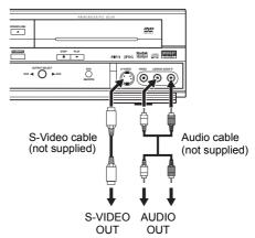
When connecting an external device of monaural output to this unit, use AUDIO L jack of AV3.
