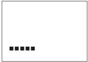
After the unit has been in pause mode for 5 minutes, it will stop automatically to protect the tape and the video head from damage.
