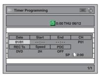
4 Enter the time to start and to end using  $[\blacktriangle / \blacktriangledown]$ , then press  $[\blacktriangleright]$ .
