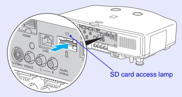
2 Remove the SD card by pulling it straight out.
