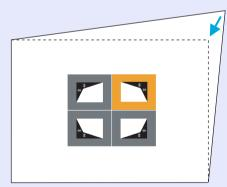
If the screen below is displayed during the correction, this means that you have reached the correction amount limit.
