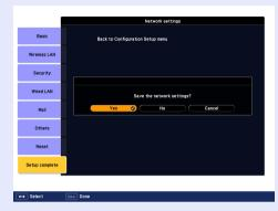
This completes the setup of the connection between the projector and the access point. Press the [Menu] button to close the configuration menu.
