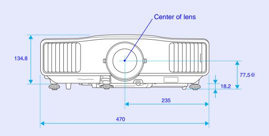
\* Distance from center of lens to suspension bracket fixing point
