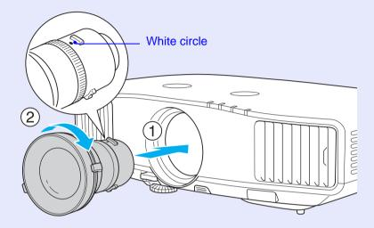
Check that the lens cannot be detached by turning it anti-clockwise.
