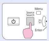
When two or more pieces of equipment are connected, press the [Source Search] button until the target image is projected.
