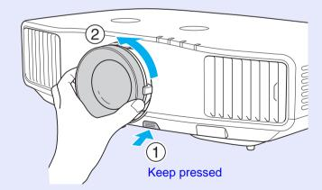
Remove the lens unit by pulling it straight out.
