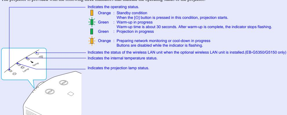
Refer to the following table to see what the indicators mean and how to remedy problems that they indicate. If all indicators are off, check that the power cable is connected correctly and that the power is being supplied normally. Sometimes, when the power cable is unplugged, the [ $\emptyset$ ] indicator remains lit for a short period, this is not a fault.
