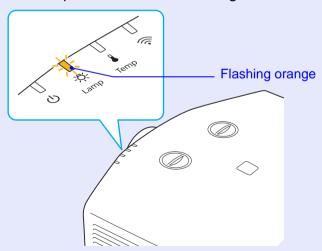
• The projected image gets darker or starts to deteriorate.
