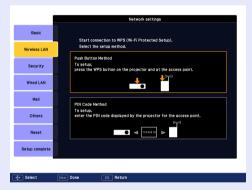
When connecting using the Push Button Method, follow the steps given below.
