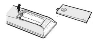
2. Insert two AA batteries. Use the (+) and (-) marks to guide you. The (+) marks on your batteries correspond to the (+) marks on the compartment. The (-) marks on your battery correspond to the (-) marks on the compartment.
