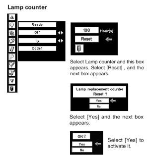
NOTE: Do not reset the Lamp Replace Counter until after the Projection Lamp is replaced.
