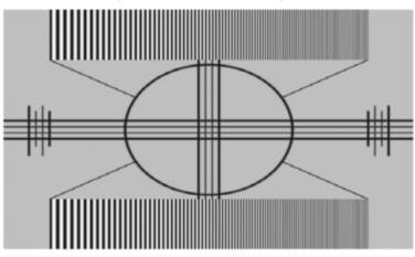
3. Adjust as needed, looking for white edges around the transitions from black to gray and differentlysized lines in the "sweep" patterns at the top and bottom. Lower the sharpness setting to eliminate them.
