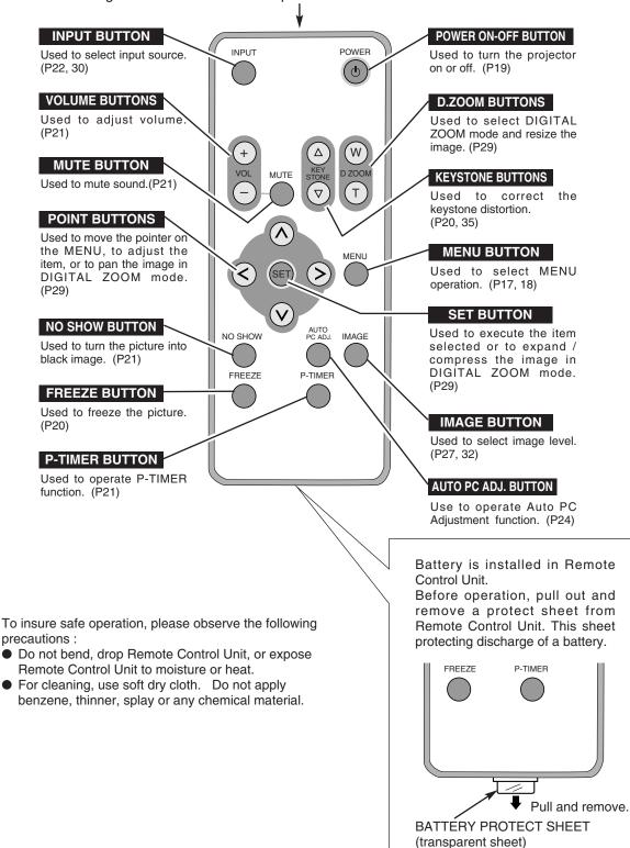
Infrared signals transmitted from this point.
